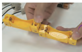
Connecting battery holders in series.
